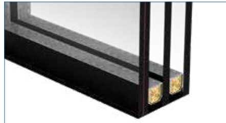
3-glass packet 44.2/12/6/12/6 SILENCE AND SECURITY
